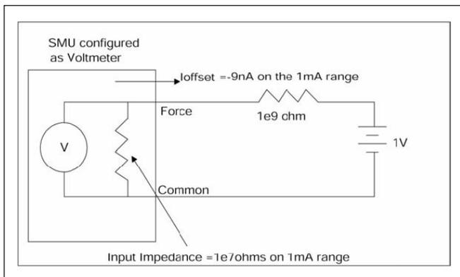
Figure 9: Mis-setting the current range to 1mA gives an input impedance of  $10M\Omega$ , which loads down the circuit under test. In addition, it allows a  $-9nA$  offset current.
