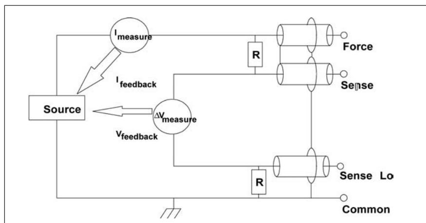
*Figure 1: An SMU includes a precision voltage source and a precision current source (shown here as one block), a voltmeter, and an ammeter.*
