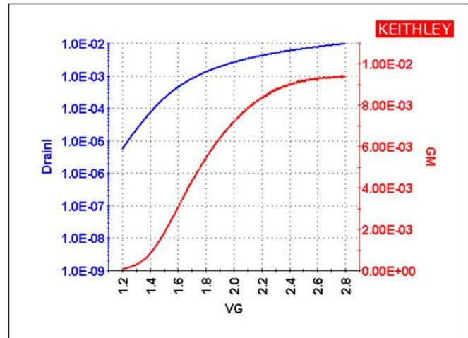
Figure 7: Floating the gate SMU on top of an extra SMU makes it possible to use the 2V range, reducing gate voltage error for error-free results.
