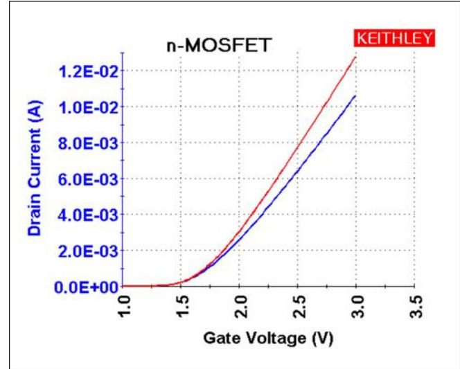
Figure 13: Connecting the SMU's Sense lead as shown in Figure 12 corrects the error.
