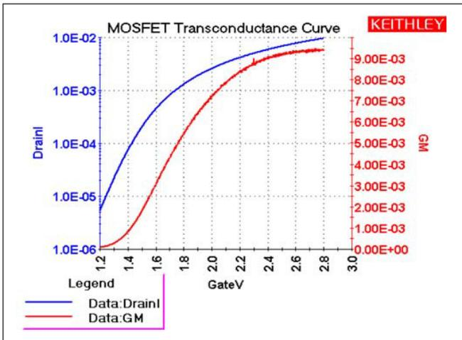
Figure 5: Differentiating the drain current with respect to the gate voltage gives an accurate result.
