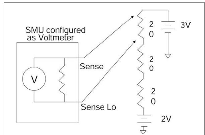
Figure 11: Measuring the voltages across these resistors is best done with a floating differential voltmeter
