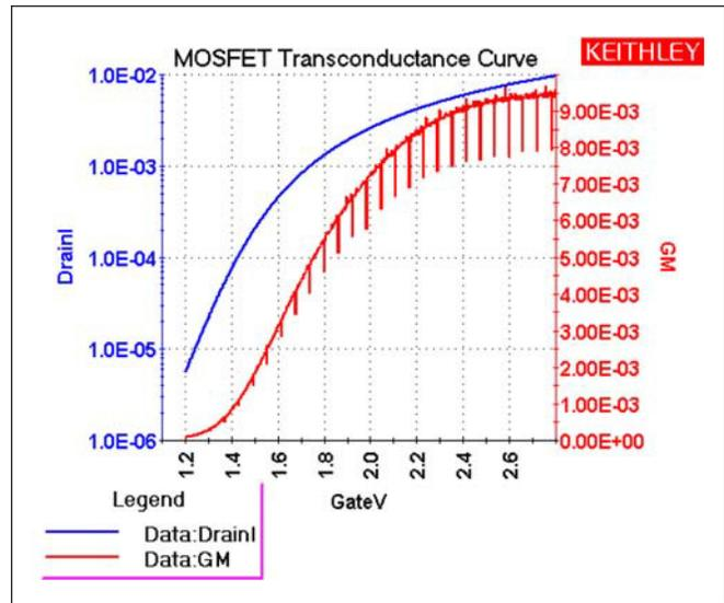
*Figure 2: MOSFET drain current (blue) and transconductance (red) curves obtained by increasing the gate voltage in 2mV steps. Note the errors in the transconductance.*
