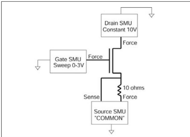
Figure 12: Connecting the SMU as shown can compensate for the drop across the source resistor.
