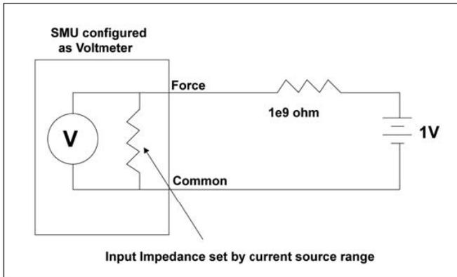
Figure 8: The input impedance of an SMU configured as a voltmeter is the reciprocal of the current range.
