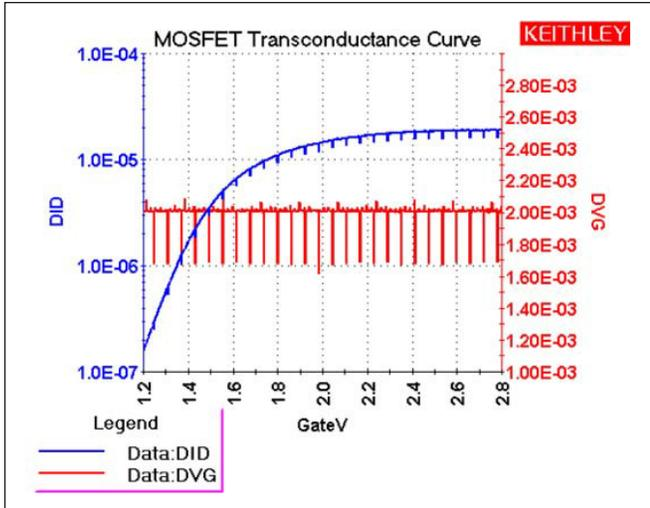
Figure 4: Measuring gate voltage with the SMU's voltmeter function reveals the cause of the problem: 300µV errors in the gate voltage.
