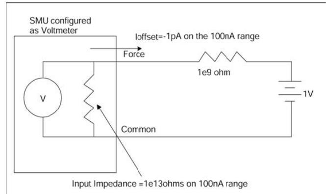
Figure 10: Setting the SMU correctly gives  $10G\Omega$  input impedance and  $-1pA$  offset current.
